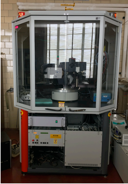
Figure 7. Bruker APEX CCD diffractometer, left, and STOE STADI P diffractometer, right.
