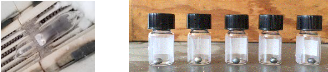
Figure 4. Tantalum ampule sealed in fused silica, left. Arc melted samples, right.
