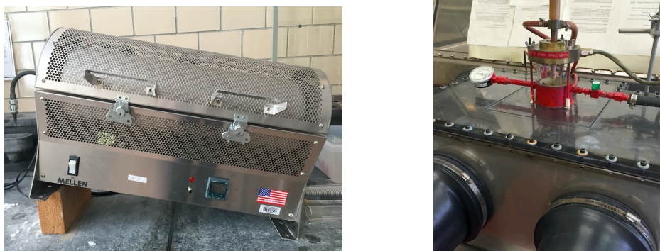
Figure 6. Mellen tube furnace with Eurotherm temperature control, left, and arc welder, right.
