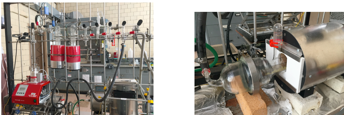
Figure 5. Schlenk line, left. Decomposition apparatus in furnace, right.
