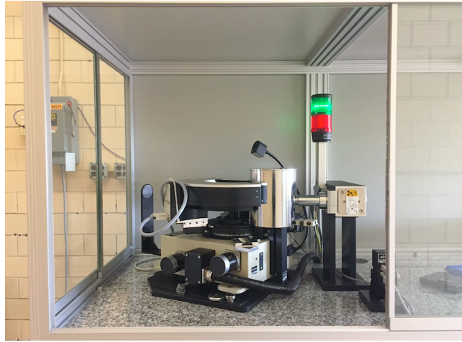
Figure 7. Bruker APEX CCD diffractometer, left, and STOE STADI P diffractometer, right.
